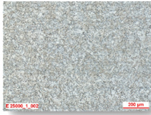
transversal section, drawn to 36.0 mm, sample taken on mid radius, Nital etching
